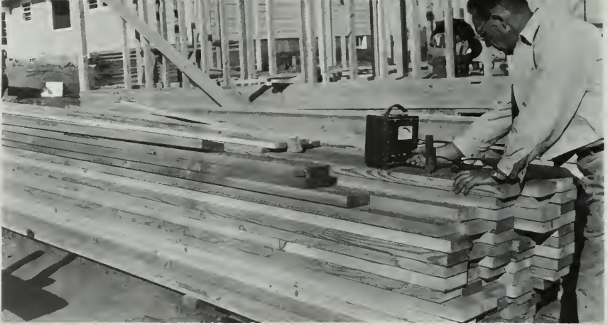
Moisture meters developed at the Forest Products Laboratory make it possible to determine whether lumber has been seasoned properly.
